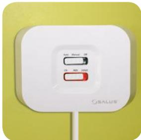
The bottom switch will show a constant red light when the iT500RX Receiver is ready to pair.
