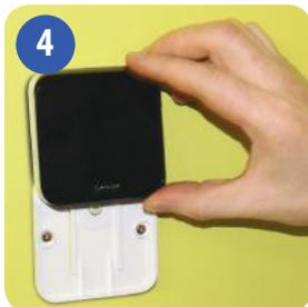
4 Align the grooves on the back of the iT300 unit and slide onto the bracket.
