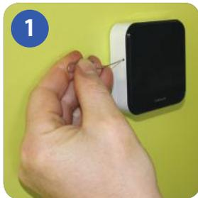
To pair the iT300 to the receiver, insert a paperclip or similar object into the hole on the left hand side of the iT300 for 2 seconds.
