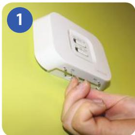
Using a paper clip, insert into the hole marked SYNC at the bottom of the iT500RX Receiver. Then work through the screen sequence shown on the next page.
