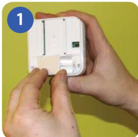
1 Remove the battery cover on the back of the iT300 unit.
