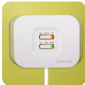
**FAILSAFE MODE:** In the event of RF signal loss, your system will be switched on for 4 minutes, then off for 11 minutes. If you want to disable FAILSAFE MODE when RF link has been lost then move the slide switch on the iT500RX to either the manual or off position.
