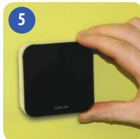
5 Once in place, ensure the unit is securely seated on the bracket.
